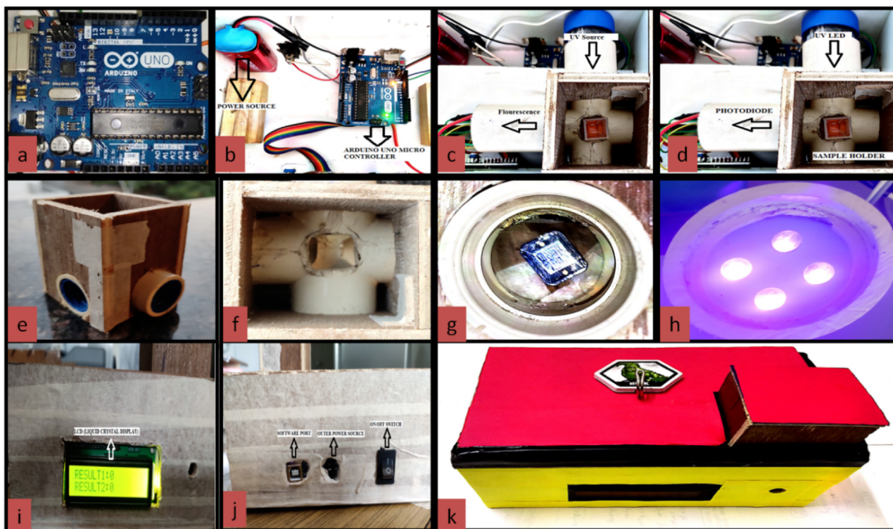
Fig. 2. Schematic representation of fabrication of device a) Arduino Uno microcontroller b) Microcontroller attached with battery source (c), (d) UV source, sample holder, fluorescence detector e), f) Design of sample holder g) Photodiode h) UV LED i) LCD for display of result j) ON/OFF switch, software update port, port for outer power source k) Final prepared prototype biosensor.
