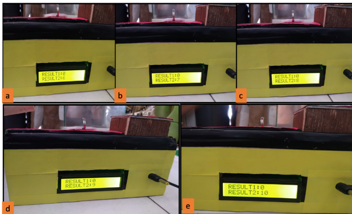
Fig. 8. Photographic image of the device showing result for a) 100 \mu\text{L} of CdTe-MPA QDs with 100 cfu b) 100 \mu\text{L} of CdTe-MPA QDs with 200 cfu c) 100 \mu\text{L} of CdTe MPA QDs with 300 cfu d) 100 \mu\text{L} of CdTe-MPA QDs with 400 cfu and e) 100 \mu\text{L} of CdTe-MPA QDs with 500 cfu.
